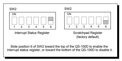
Figure 8--- Enabling the Interrupt Status Register
